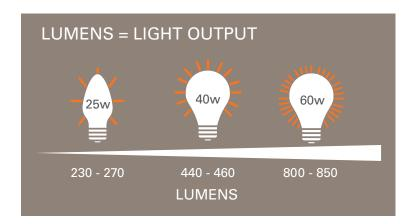
For non-directional bulbs, such as a globe or candelabra, the total lumen output is calculated in all directions. With a directional bulb, such as a spotlight, the light is emitted in many directions, some of the light (spill light) may not be useful but it is counted in the total lumen rating.
