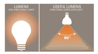
Useful lumen rating is a measurement of useful light emitted in a standardized 90-degree cone. The useful lumen rating is usually lower than the total lumen output but has more relevance to a spotlight bulb where useful light is in a forward focused direction.
